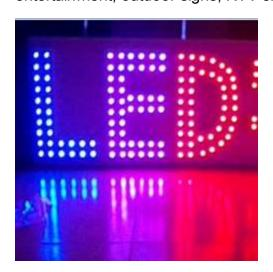
RGB Pixels are digitally-controllable lights you can set to any color, or animate. Each RGB LED and controller chip is molded into a 'dot' of silicone. The dots are waterproof and rugged. There are four flanges molded in so that you can 'push' them into a 12mm drill hole in any material up to 1.5mm/0.06"
